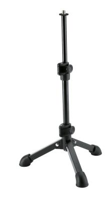
The telescopic microphone stand with a 3/8" threaded connector is extremely versatile. Its height can be adjusted from 230 to 400 mm using the practical clamping lever. This light-weight three-legged stand with folding legs is suitable for mobile operation. The robust foot end caps provide stability and reduce undesirable transmission noise.
